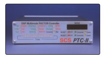
proven with a 16 <u>milliwatt</u> link between Europe and Australia! The PTC-II is fully backwards compatible with all known PACTOR I implementations.
